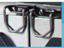
The door locking mechanism has an integrated two-point lock which holds the doors securely closed, even on rough or uneven surfaces. The doors can be opened using one hand.
